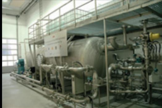
MPM includes flow tests as part of the standard Factory Acceptance Test, and offers training of field operators at the unique MPM Flow Laboratory. It is made to enable testing of flow meters at field simulated conditions, and has highly accurate reference instrumentation.
